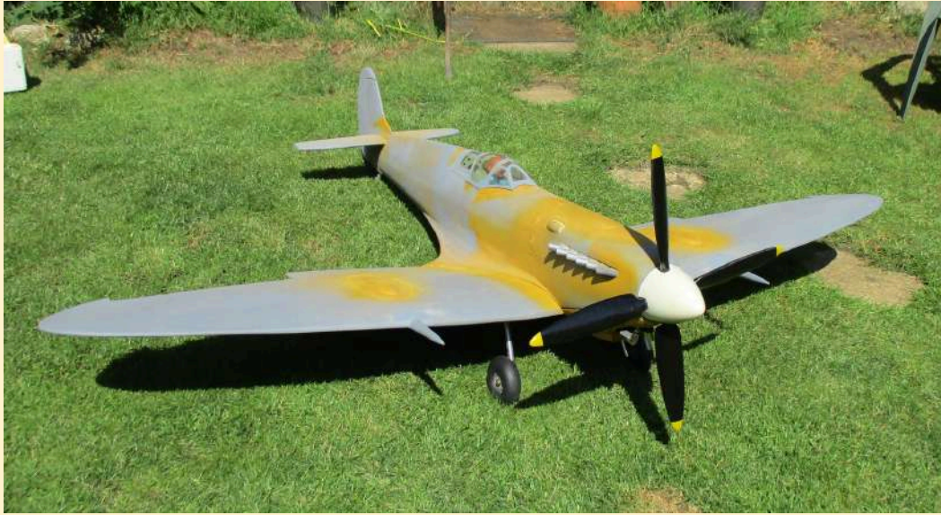
More primer, scale propeller, cannons, wing blisters and canopy added, 17/06/2017
