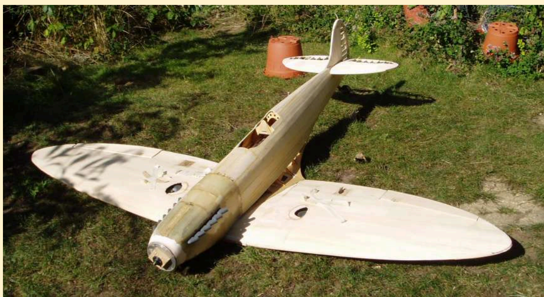
Most of the structure was complete in 2013 and nearly ready for fibre glass cloth covering
